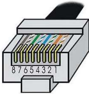
Fig 5.1 Pin Configuration for standard Type T-568B RJ45 plug
