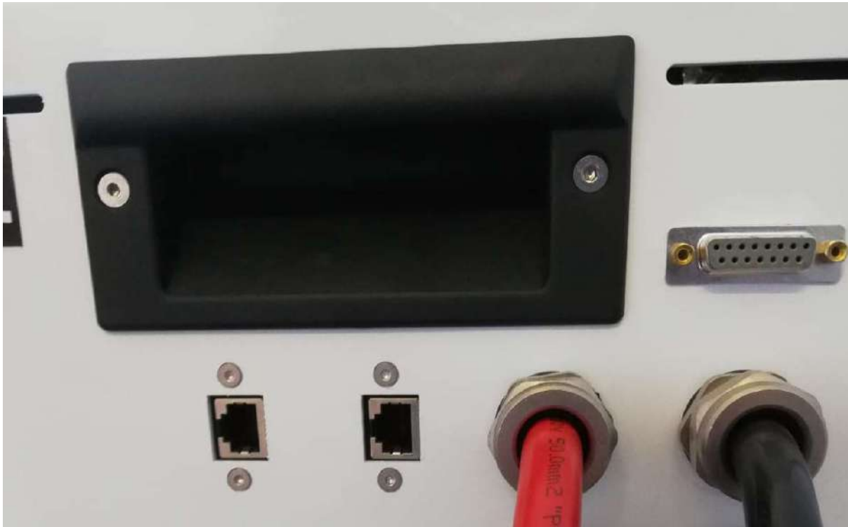
Figure 5.2 Picture Showing 2 x RJ45 Sockets for CAN Bus (DB15 Plug shown here for Analogue and Relay Control is not available in new models)
